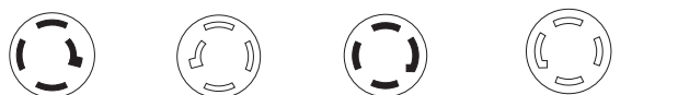
PLUG NON-NEMA 20A 120/208V 3ØY RECEPTACLE NON-NEMA 20A 120/208V 3ØY PLUG NON-NEMA 30A 120/208V 3ØY RECEPTACLE NON-NEMA 30A 120/208V 3ØY
