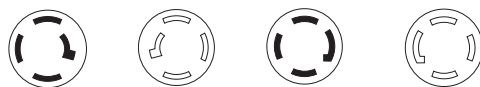
PLUG NON-NEMA 20A 120/208V 3ØY RECEPTACLE NON-NEMA 20A 120/208V 3ØY PLUG NON-NEMA 30A 120/208V 3ØY RECEPTACLE NON-NEMA 30A 120/208V 3ØY
