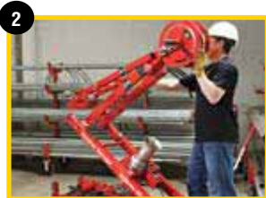
Flip booms into position and lock
