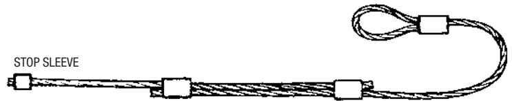
LAP SPLICE - OVAL SLEEVES OR DUPLEX
