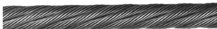
Left Lang Lay – Strands are laid to the left but wires appear to make an angle with the rope.
