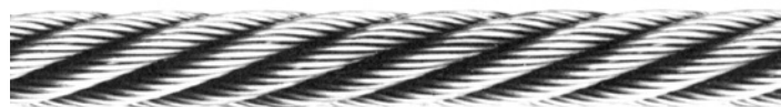
Left Regular Lay – Strands are laid to the left and wires appear in line with the rope.
