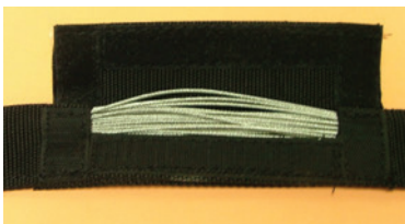
Velcro inspection window
