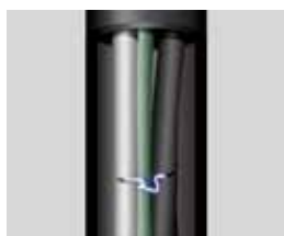
Parallel Arc Fault
