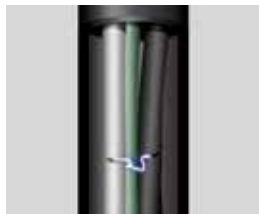
Parallel Arc Fault
