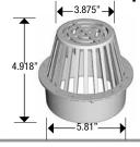
**Use with:** 6" round basin, 6" corrugated singlewall pipe or 6" SDR 35 pipe where debris would clog a flat grate.
