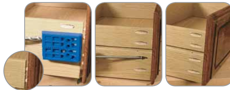
Drill Pocket-Holes at the problem joint.
