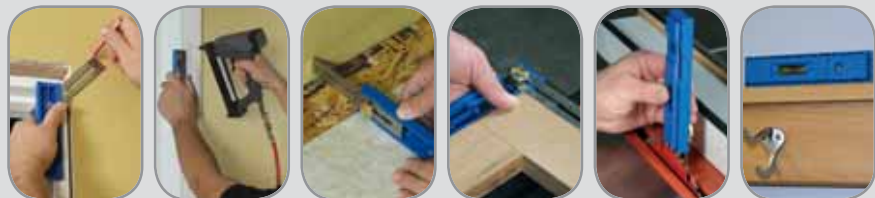
Layout Mitered Corners Set 3/16" Reveals Transfer Measurements Align / Square Your Projects Set Bit / Blade Heights Use as a Simple Level
