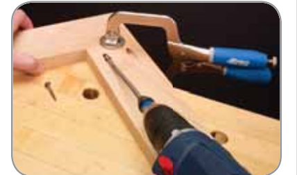
Kreg screws are available in a wide variety of lengths, as well as coarse and fine thread types, depending on the type of wood you are working with. (See more on page 17)
