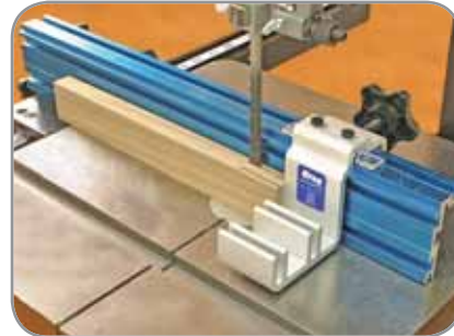
Add a stop to the fence for producing cuts to a repeatable depth, such as cutting tenons.
