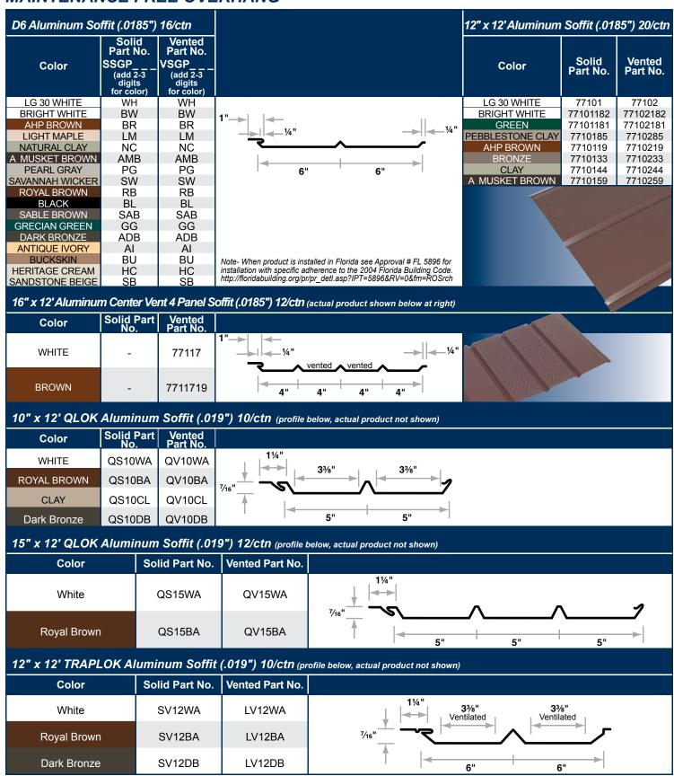
~Air Flow for Vented Soffit is 6 square inches per 1 square foot.
