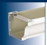
Nails or screws required. Fasten to fascia board along sloped string guide line. Place gutter into bracket, snap top bar into slot and front bracket.
