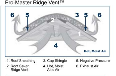
Air flow across the exterior roof ridge draws hot, moist attic air out through the Ridge Vent and pulls fresh air into the attic through the soffit vents. Removal of hot, moist air from the attic reduces cooling costs and eliminates potential damage to your roof.
