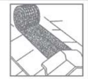
Vent must be used on roofs with a minimum 3/12 pitch.
