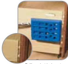
Drill pocket holes at the problem joint.
