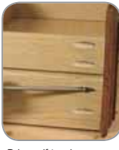
Drive self-tapping screws to secure the joint.
