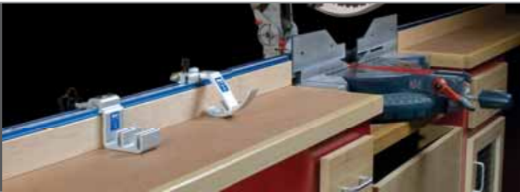
Center your saw with 4 feet (1200mm) of Trak on each side.
