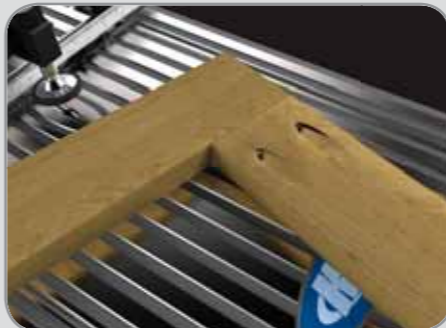
DRILLS ALL 3 KREG JOINTS The all-new Foreman is the first Kreg Pocket-Hole Machine that can drill all three types of Kreg Joints: Standard for materials from ½" (12mm) to 1½" (38mm) thick, Micro-Pocket™ to create more compact pocket holes in thinner stock, and HD (Heavy-Duty) for creating strong joints in 1½" (38mm) and thicker stock.
