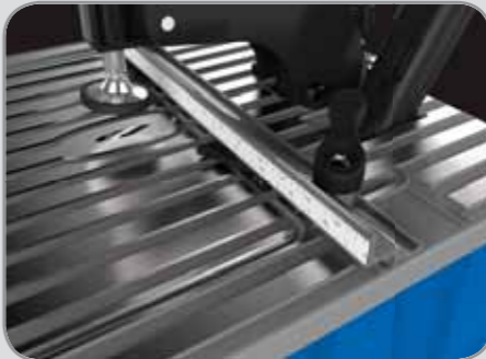
ADJUSTABLE FENCE & STOPS To ensure perfect pocket-hole placement, the Foreman features a tool-free adjustable fence that positions your workpiece for precise pocket depth, and a pair of adjustable, spring-loaded stops that provide repeatable accuracy.
