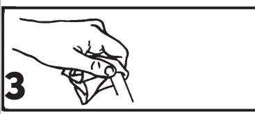
Fig. 1 Using Genova Plastic Tubing Cutters (PN 53499), cut tubing squarely to length.
