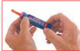
2. Turn dial to expose 1/8" to 1/4" of material beyond tip.
