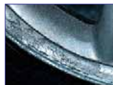
Curbside Rash & Scuffs
