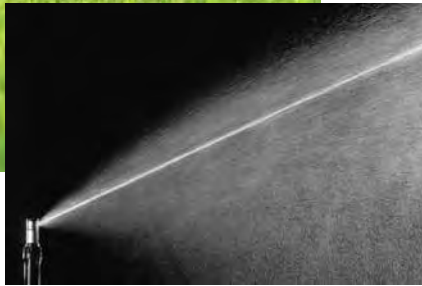
Competitive rotor with uneven water delivery
