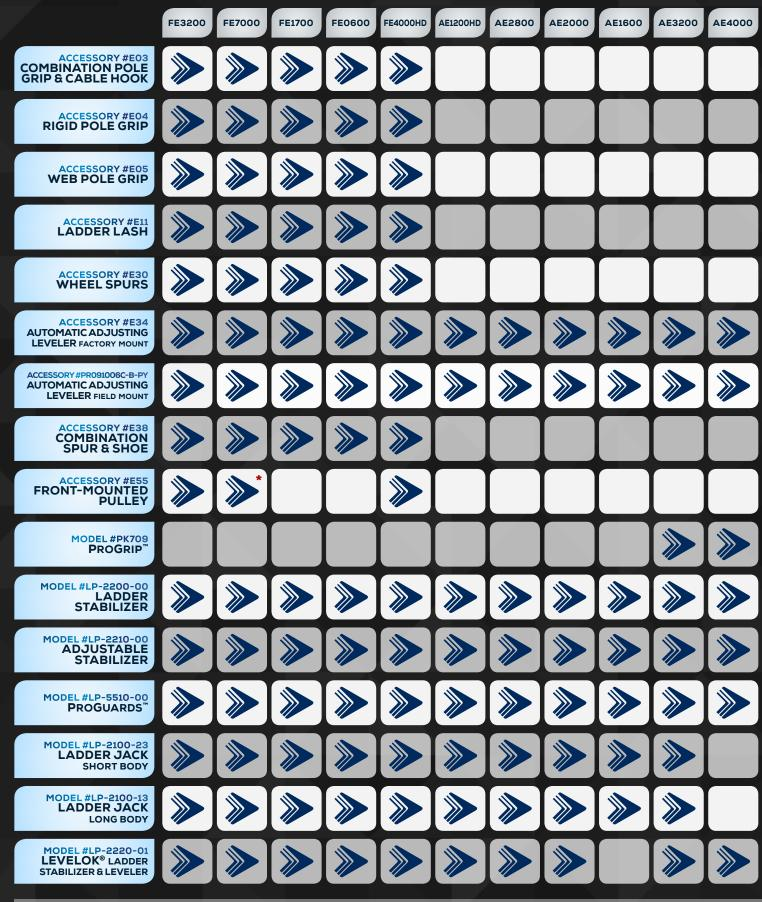
For availability, please contact Customer Service. Specify ladder size and model. To order factory-mount accessories, add the 3-digit accessory number and size. EXAMPLE: FE3220-E05, 20' Fiberglass Extension Ladder with Web Pole Grip. \*Only fits 16'-32' models
