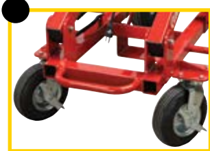
G Swiveling casters/ mobility • Moves easily on dirt and gravel • Flat-free wheels
