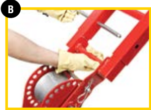
B Extended boom • Allows 12' of cable to be pulled from the conduit to the capstan
