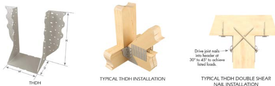
FIGURE 9—THDH FACE MOUNT HANGER
