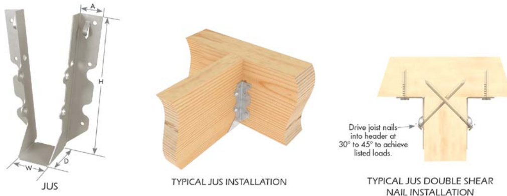
FIGURE 6—JUS SLANT NAIL JOIST HANGER
