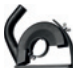
Protective suction hood with guide block for cutting discs Ø 230 mm cutting depth 65 mm, connection Ø 32 mm
