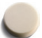
Polishing sponge For polishing painted surfaces. Various hardness grades: soft for new paintwork, medium for slightly weathered paintwork and applying wax, hard for severely weathered paintwork. Quick hook and loop fastening, height 40 mm.
