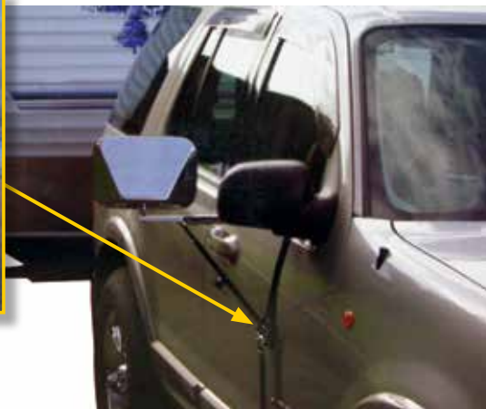
Rubber pad protects vehicle's finish
