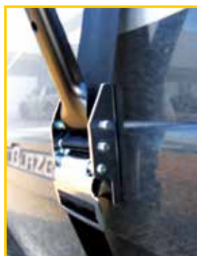
Rubber pad protects vehicle's finish
