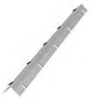
The TradeReady<sup>®</sup> Spazzer<sup>®</sup> 9200 bar is a pre-notched, 20 gauge, galvanized steel spacer and bridging bar. It facilitates rapid erection of studs into a rigid, accurately laid out gridwork that has excellent resistance to stud rotation and displacement. Hanging drywall is also faster and easier because the Spazzer 9200 bar eliminates the bow that often occurs in tall interior studs.
