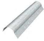
ClarkDietrich kerfed bullnose has a distinctive shortened back flange allowing for insertion into grooved door jambs and window trims. This feature provides for efficient, clean installation, as well as the smooth round appearance associated with bullnose trims. Roll-formed from galvanized steel, it conforms to ASTM C1047 for added durability and protection from corrosion.
