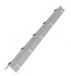
The TradeReady<sup>®</sup> Spazzer<sup>®</sup> 9200 bar is a pre-notched, 20 gauge, galvanized steel spacer and bridging bar. It facilitates rapid erection of studs into a rigid, accurately laid out gridwork that has excellent resistance to stud rotation and displacement. Hanging drywall is also faster and easier because the Spazzer 9200 bar eliminates the bow that often occurs in tall interior studs.
