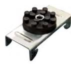
The RSIC-1<sup>®</sup> resilient sound isolation clip is used in conjunction with drywall furring channel to fasten gypsum wallboard to various wall and floor-ceiling designs and applications, while simultaneously providing acoustical separation (decoupling). This significantly reduces the amount of impact and sound that filters from surrounding rooms-reducing the noise transfer by 75 to 100%.
