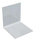
ClarkDietrich aluminum burn clips are used as part of the H-stud area separation wall assembly and are designed to melt when exposed to fire. The clips hold the area separation wall assembly in place at the floor, roof and truss line between adjacent units. In a fire, the aluminum burn clips on the fire-ridden side of the wall will melt, allowing the wall structure for that side to collapse.
