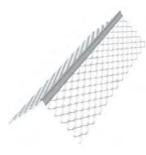
ClarkDietrich 1A expanded flange corner bead is used to provide strong corner reinforcement for conventional plaster applications. A solid metal nose provides a straight, rigid ground for screeding, and the 2-7/8" or 3" flanges can be flexed easily over irregular, uneven surfaces. Plaster keys near the solid nose provide increased reinforcement where needed and ensure straight corners.
