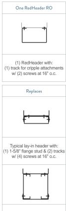
Typical boxed header with: (2) 1-5/8" flange studs & (2) tracks w/ (4) screws at 16" o.c.
