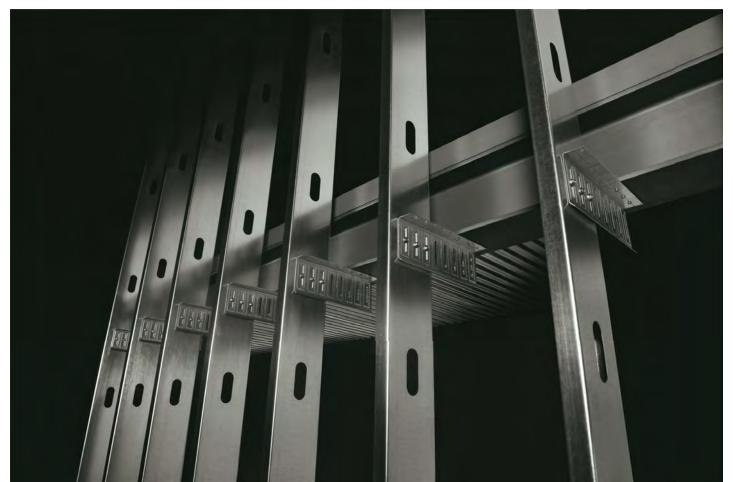
ClarkDietrich FastClip™ slide clip deflection clips are used to attach exterior curtain wall studs to the building structure and provide for vertical building movement
