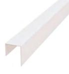
provides a finished edge at gypsum board stops around door and window openings and at ceiling intersections. Requires no joint compound. Rigid vinyl is not a thermal transmitter and helps stop condensation where gypsum board terminates at exterior metal surfaces, such as window frames and mullions. Rustproof and dent-resistant.
