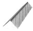
ClarkDietrich Mini-Bead™ 800 and 900 are fine-mesh corner beads used to provide corner reinforcement for one- and two-coat veneer plaster systems. Mini-Bead 800 has 1/16" grounds for one-coat veneer plaster and 90 keys per linear foot for excellent bonding and strong corners. Mini-Bead 900 has 3/32" grounds for two-coat veneer plaster systems.
