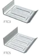
ClarkDietrich Fast Top<sup>™</sup> clips are used in head-of-wall deflection conditions for in-fill curtain wall assemblies to provide for vertical movement. These clips are used in place of, or in combination with, deflection track. They also make a positive attachment and eliminate the need to install bridging continuously throughout the uppermost punchouts. Attach to the underside of structural members, concrete decks or floor assemblies.
