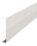
Platinum L-trims are used to finish the ends of wallboard where it abuts dissimilar surfaces, such as suspended ceilings, beams, plaster, masonry or untrimmed door and window jambs. Applied in the same manner as all other tape-on beads joint compound embeds the paperfaced bead to the wallboard paper.
