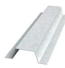
ClarkDietrich heavy-duty furring channel is a high-performance framing component used in ceiling, exterior wall and roof applications. With two standard depths—7/8" and 1-1/2"—heavyduty furring channel provides greater resistance to deflection and bending. In roof applications, heavy-duty furring is used as purlins to provide connection points for roof sheathing.
