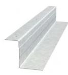
ClarkDietrich Z-furring is used to furr out interior masonry or poured concrete wall substrates and to support rigid polystyrene, mineral, or fiberglass batt insulation while providing a uniform plane for gypsum panel attachment. Z-furring should be installed vertically with the 3/4" flange against the substrate. The type of fastener and spacing will vary based on application. Install gypsum wallboard parallel or perpendicular to Z-furring.
