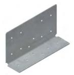
SwiftClip<sup>™</sup> L-Series<sup>™</sup> support clips are used in multiple construction projects, specifically in conjunction with structural studs and track. The L-shaped clips fit between the stud flanges, so that shorter length clips do not need to be ordered. These labor time-savers include prepunched holes for quicker screw attachments, and are punched to accommodate for CRC lateral bracing connections.
