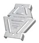
The ClarkDietrich FastBridge<sup>™</sup> Clip is used to secure 1-1/2" U-channel [Cold Rolled Channel (CRC)] to structural wall studs when used in load-bearing or curtain wall applications. The wall stud friction fit design allows for as little as one screw for the connection to the U-channel. Do not use in studs over 8" wide.
