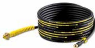
The pipe cleaner uses four backward firing high pressure water jets to propel itself through pipes to break up and evacuate built-up debris and grime. The kink resistant flexible hose includes measurement markings and a ring to indicate progress. Connect directly to the trigger gun.
