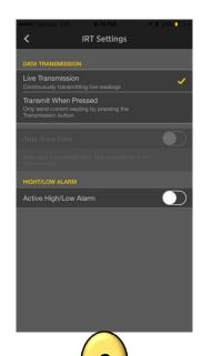
The default settings are set as "Live Transmission" with active high/low alarm turned off. Tap the Save button on the infrared thermometer's dashboard to save a transmitted value to the databank.
