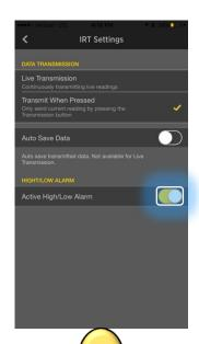
Click the "Active High/Low Alarm" button to turn on a custom range to notify you when a value falls within or outside of the range.
