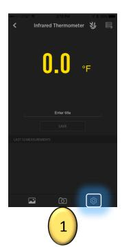
From the dashboard, tap the settings button in the bottom right corner of the screen to access the infrared thermometer's settings
