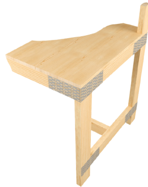
Typical mending plate installation
