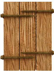
WS35 installed in (3) 1-3/4" Ply
