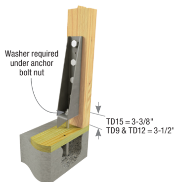
Typical TD15 installation
