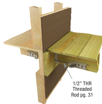
Typical DTB-TZ deck to ledger installation
