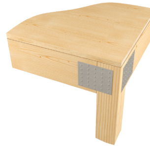
Typical nail plate installation
