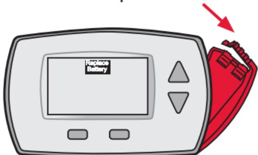
Insert fresh AA alkaline batteries, then reinstall battery holder.
