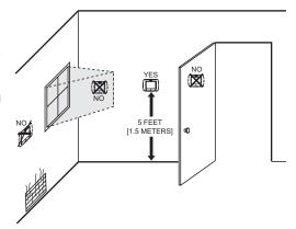
Fig. 1. Selecting thermostat location.
